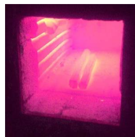
Figure 3.1 Soaking of raw samples at 900°C for 4hrs
